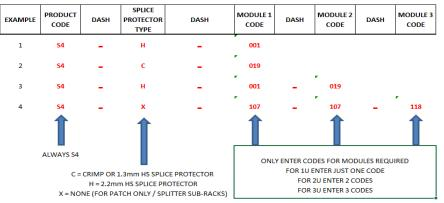
**Example 1** above is for a 1U SRS Sub-Rack. The part number is S4-H-001. This denotes a 1U high SRS4000 Sub-Rack fitted with a blank Splice and Patch module. The sub-rack is for use with 2.2mm heat shrink splice protectors.
