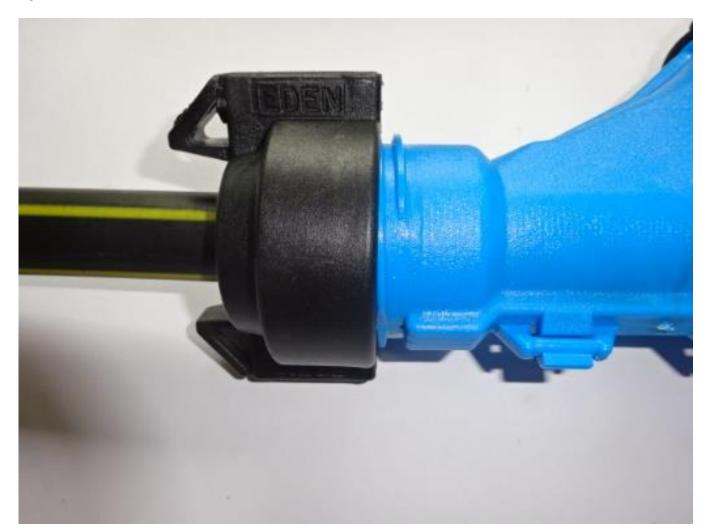
Tighten the input locking nut.
