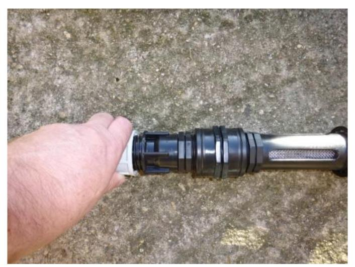
Tighten the lock nut to secure the SDMB Guard 1.
