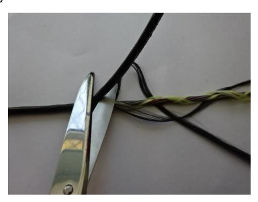
Remove the cable sheath.
