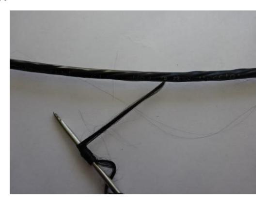
Using one of the rip cords apply a longitudinal cut to the mark in Step 2.
