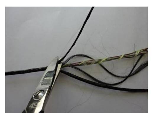
Remove the split cable sheath.
