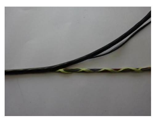
Remove the cable core from the sheath.
