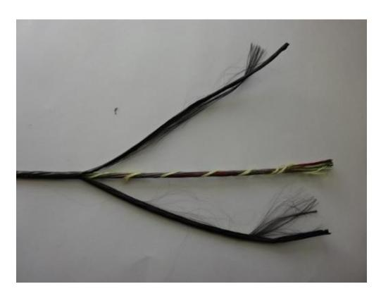
Separate the cable sheath.
