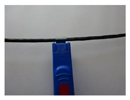
On a dummy section of cable determine the setting of the cutter to ensure that the depth of the cut does not damage the tubes.
