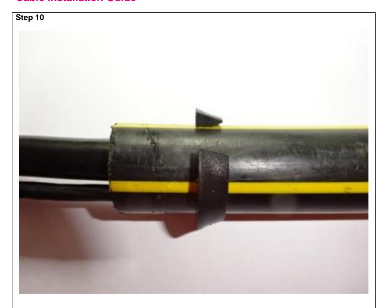
On one of the closures position the SDMB5 Grab Ring onto the sub-duct. Note the orientation! The front face of the Grab Ring should be 25mm from the end of the SDMB5.
