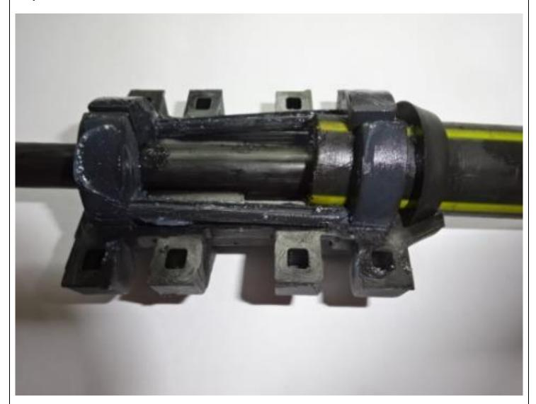
Position the seal within the bottom half of the closure.
