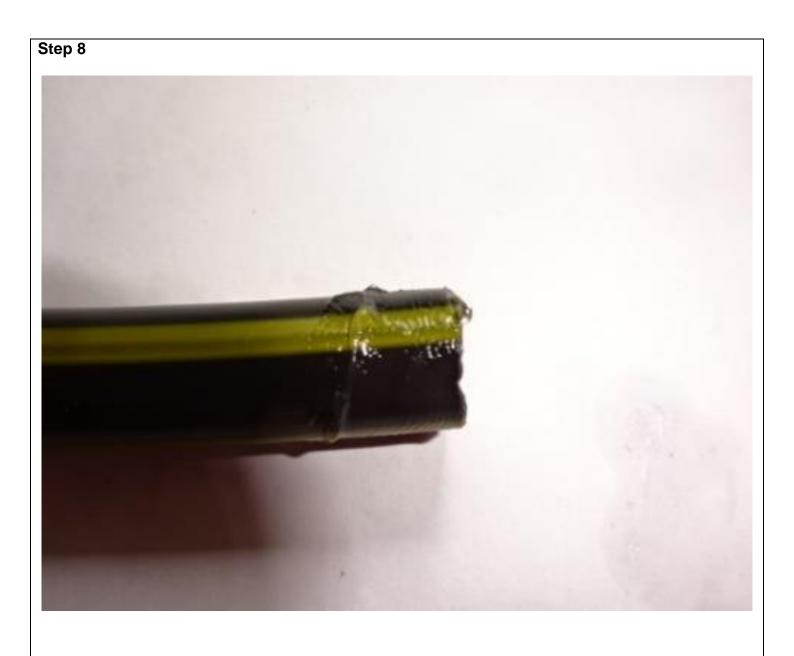
Smear some silicone grease around the bottom of the mini-ducts.
