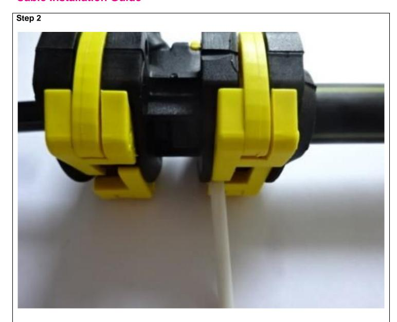
Using the toggle release tool release the toggle.
