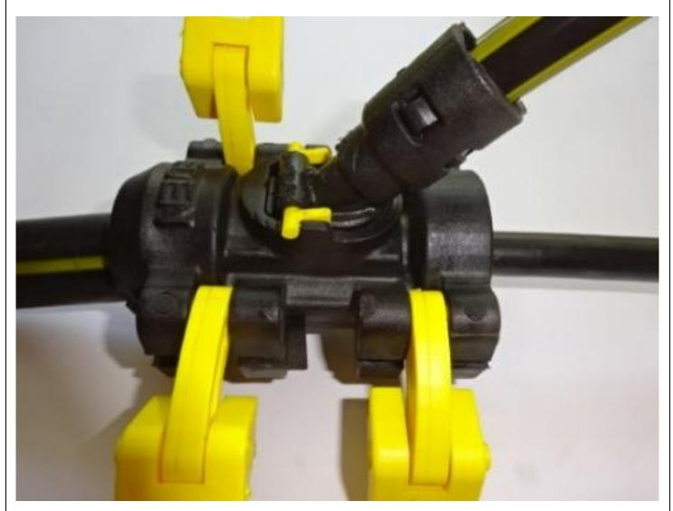
Carefully position the top half of the closure body over the bottom half.
