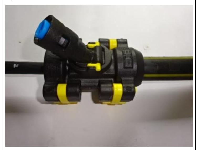
Seal the closure using the toggle clamps.
