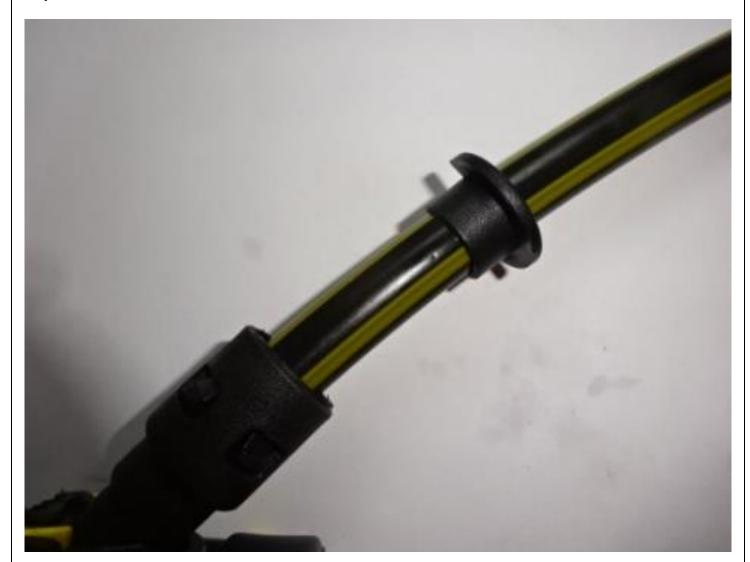
Clip the Mini-duct Release Tool over the 14/10mm mini-duct.
