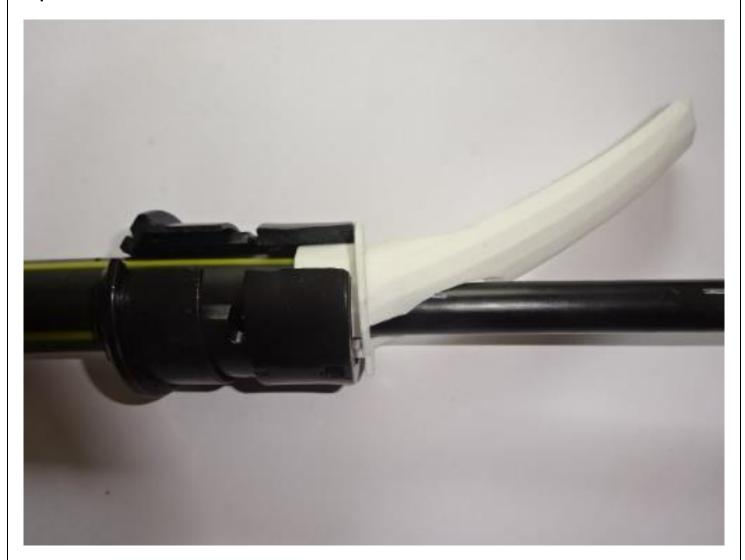
Fit the deflector plate onto the end of the sub-duct and position in the grab ring.
