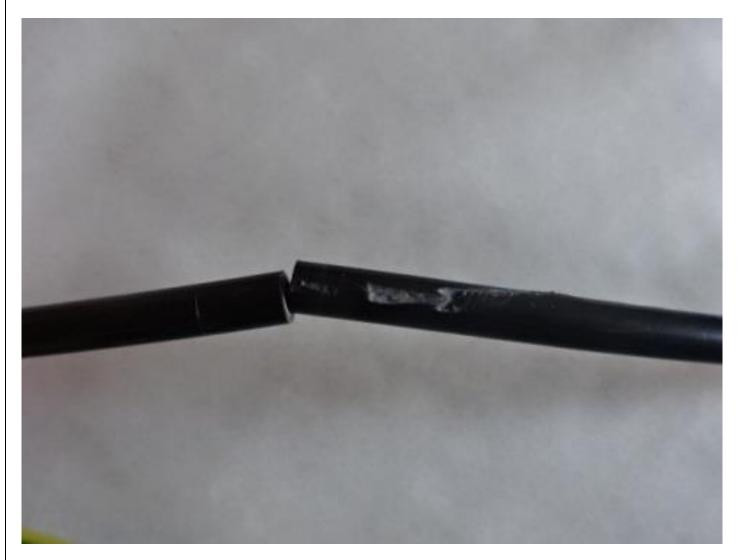
At the relevant position apply a circumferential cut to the tube and flex the cut. Remove the section of tube.
