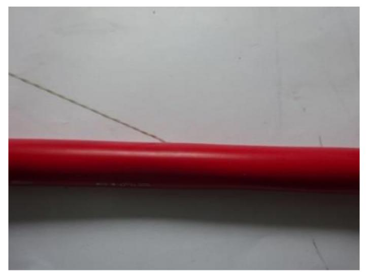
Using the rip cords apply two longitudinal cuts to the cable sheath to the mark identified in Step 2.
