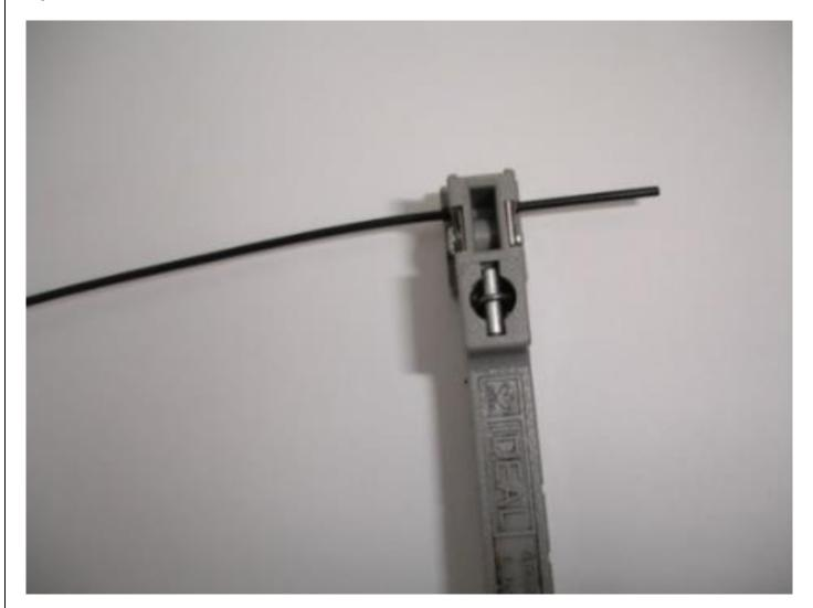
On a scrap section of unit set the depth of cut for the longitudinal and circumferential cutters.
