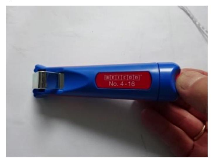
Adjust the cutter depth to ensure that the blade cuts through the cable sheath.
