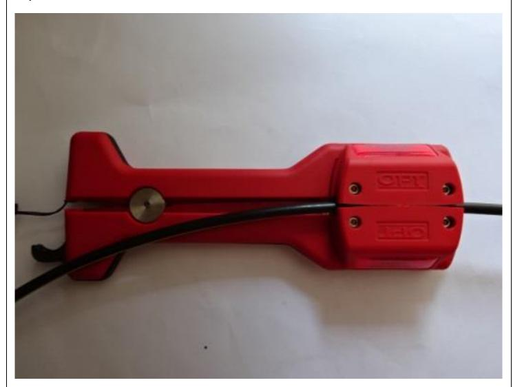
Assemble the Sheath Cutter around the cable at this point.
