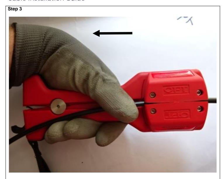
Pull the Sheath Cutter along the cable towards the free end of the cable.
