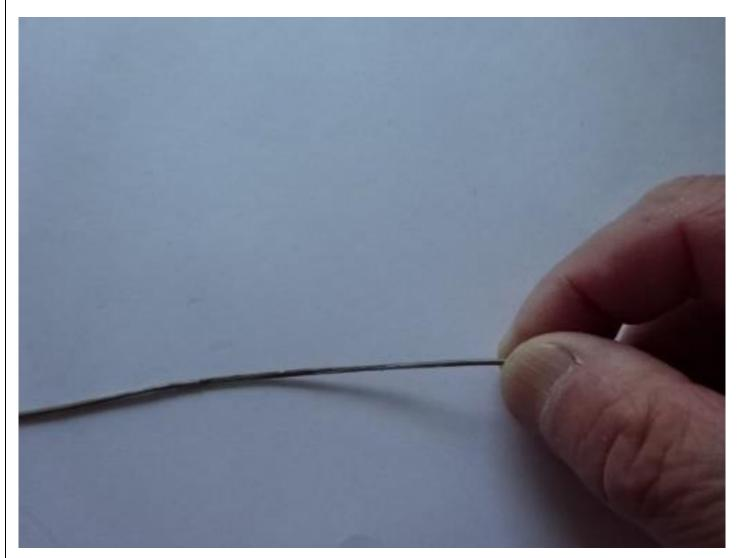
Remove the tube from around the optical fibres.
