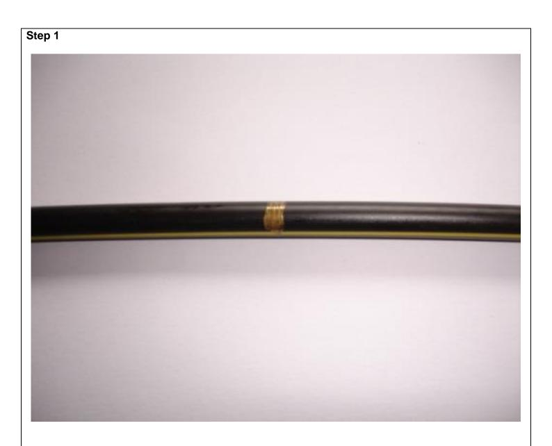
Determine the amount of cable sheath to be removed and mark the cable sheath at the required points.
