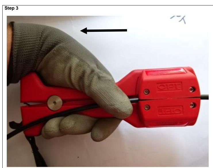
Pull the Sheath Cutter along the cable towards the free end of the cable.
