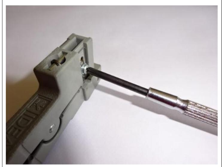
If required adjust the cutter depth to ensure that the optical fibres are not damaged.
