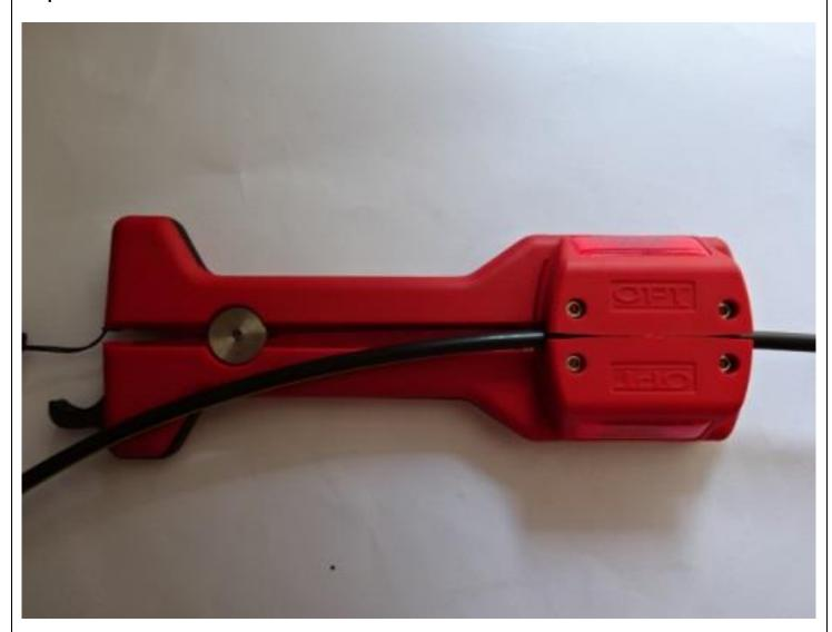
Assemble the Sheath Cutter around the cable at one of these point.
