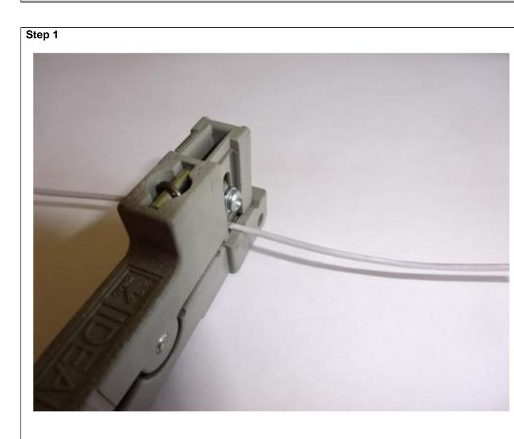
On a sample of tube check the setting of the peg cutter to ensure that the optical fibres are not damaged by the operation of the cutter.
