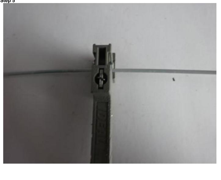
At a position 500mm from the end of the tube apply a circumferential cut.
