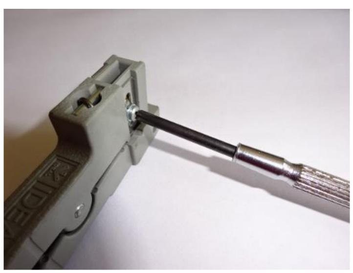
If required adjust the cutter depth to ensure that the optical fibres are not damaged.
