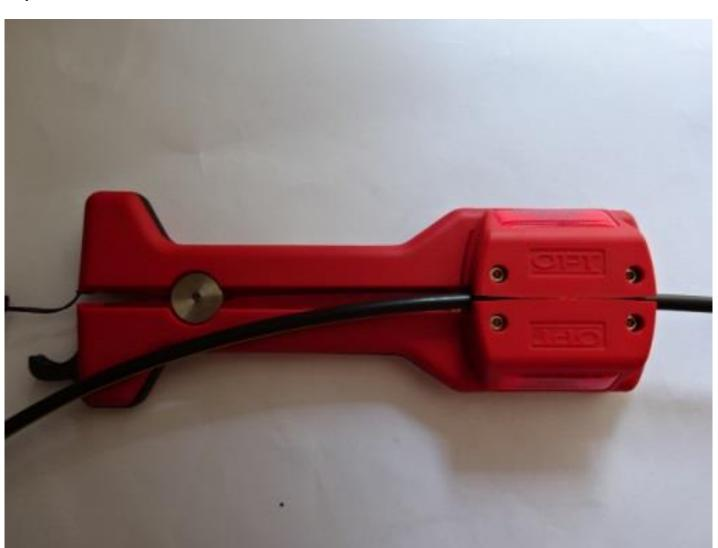
Assemble the Sheath Cutter around the cable at this point. To ensure that the cutter blades do not get damaged ensure that they are positioned on the yellow line on the cable sheath. If there is no yellow line then the blades should be positioned on the sheath printing.
