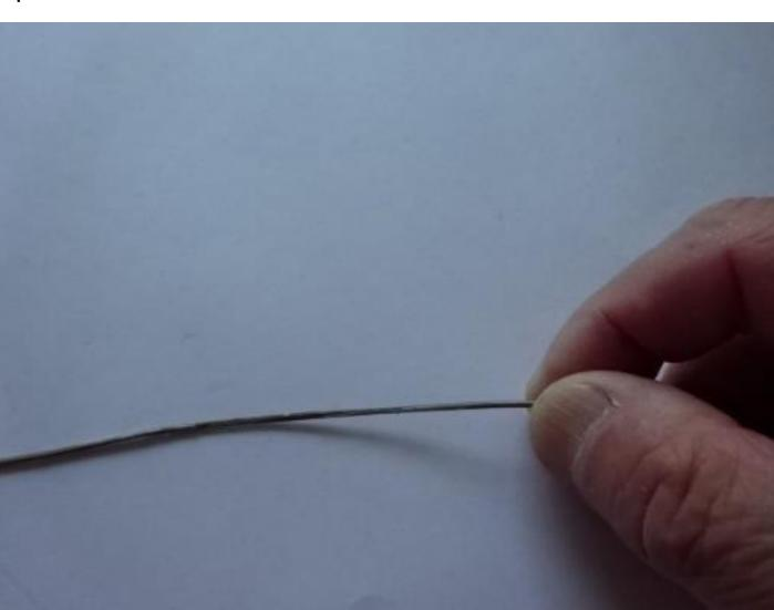
Remove the tube from around the optical fibres.
