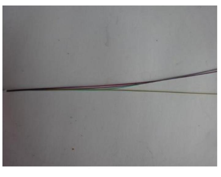
. Separate the optical fibres.
