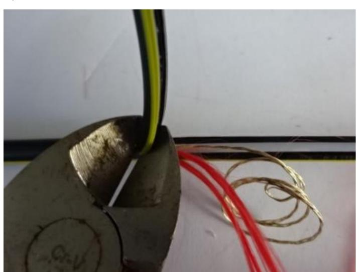
Cut the sheath at the point identified in step 1.
