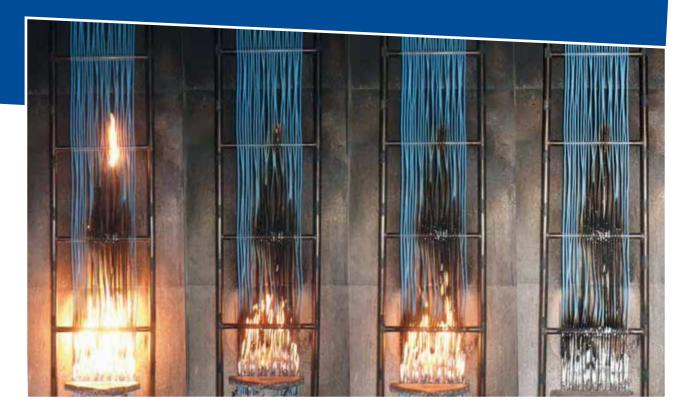
Figure 4 - Draka Category 6 U/UTP C<sub>ca</sub> D64 Cable Successfully Achieving Euroclass C<sub>ca</sub> Classifiction in a EN50399 Test
