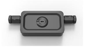
The MSB is a splice box designed for use in the external environment with an IP rating of IP68. The box houses four splices. The box has four ports which are compatible with a mechanical cable sealing system. Two are included with box. The box is deigned for cables to pass through if required. The MSB can accommodate cables with diameters from 4mm to 6mm.
