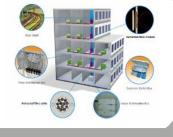
**Blowable micro-duct systems**. Simple, well established blowable solutions to fulfill the need for a flexible fibre system Enabling the customer to **scale its passive network** to the demands of end-user without high capital expenditure or extensive network planning. Fibre deployment by using **compressed air** to blow optical cables and EPFUs into microducts.
