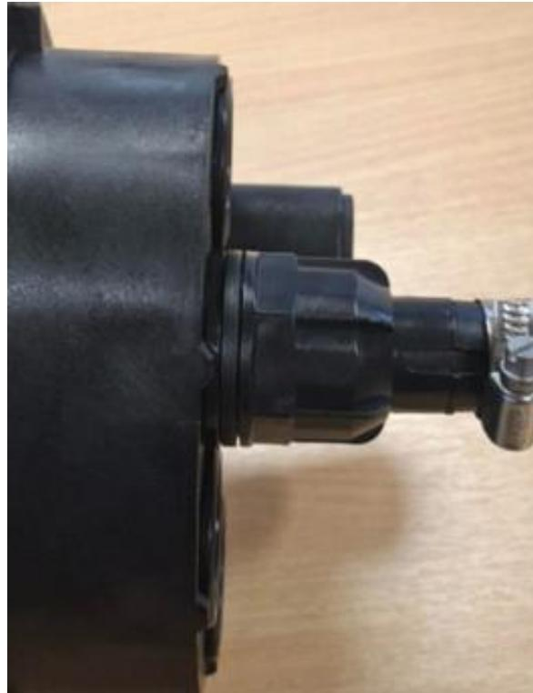
Once the gland has been assembled it can be inserted into the required port in the base. Ensure that the duct is pushed fully into the seal. A click noise can be heard when it is seated correctly.
