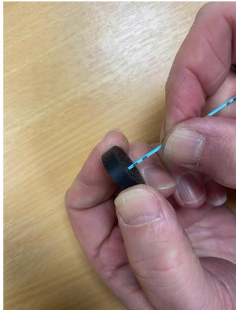
Holding the top part of the seal with the grooved face pointing outwards push the first fibre through one of the holes in the inner circle. Once this or any fibre has been pushed through do not remove the fibre. Any opened-up holes that are not used will compromise the seal.
