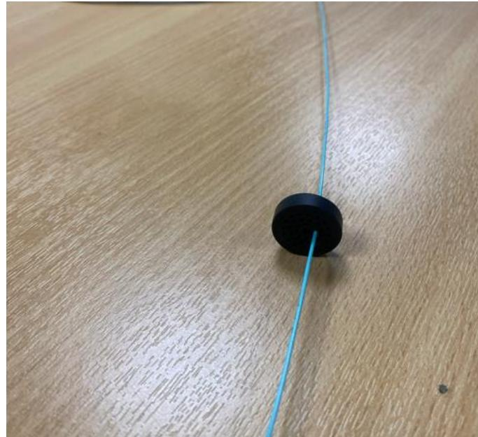
The fibre will easily push through the thin piece of rubber inside the seal. Pull the required amount of fibre through the seal.
