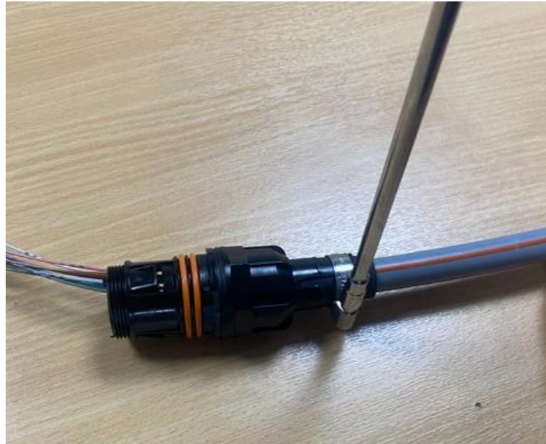
Place the jubilee clip over the end of the anti-torsion piece and rubber seal and fully tighten.
