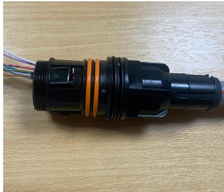
Slide the anti-torsion piece and nut up to the gland body, do not fully tighten. Ensure that the duct is fully inserted into the rubber seal and that the anti-torsion piece is locked onto the gland body and cannot turn. Now the gland nut can be fully tightened. Tighten until there is no movement in the three washers.
