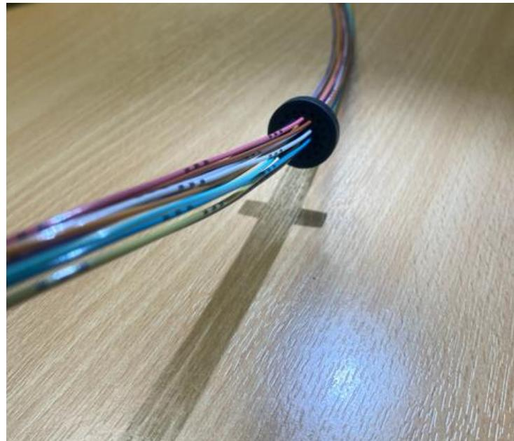
Continue pushing fibres through the holes starting from the inside group of holes and working outwards.
