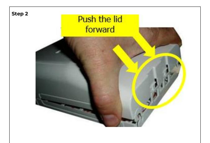
Then push the top of the lid onto the PBI-16SC and ensure that both cover clips have been clicked into place.
