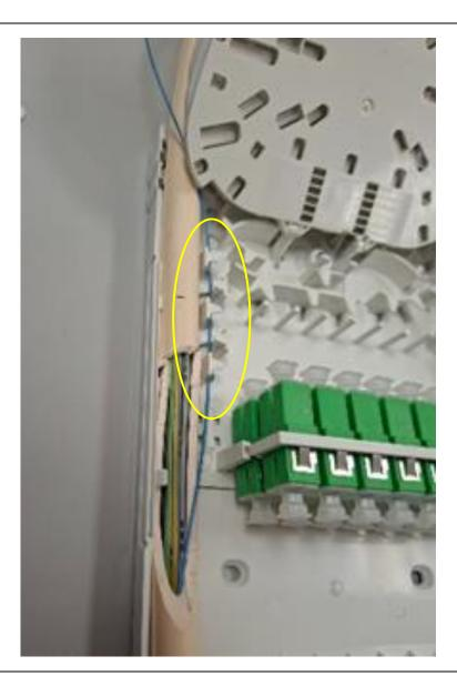
The fibers can then be routed through the PBI-16SC, using the fibre guides that are built into the PBI-16SC and will safely guide the fibers into the desired tray.
