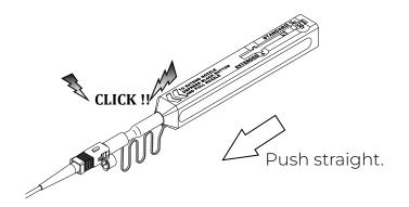
Be careful not to slant SC Connector while inserting into the Guide сар.
