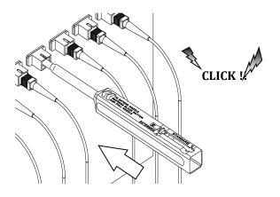
Be careful not to slant the SC Connector Cleaner while inserting into the adapter.
