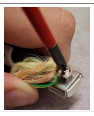
Coil the Kevlar underneath the retention bracket, go around 3 times before tightening.
