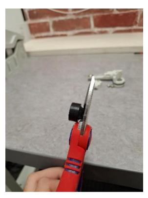
The grommet with the smaller hole is for cables that are 6mm. Medium grommet size is 8mm, whilst the large grommet is for cables of 12.5mm. After selecting the correct grommet, depending on the cable diameter, use scissors to cut the end open.
