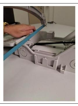
Use a saw for the hole, ensure no sharp edges or grooves remain as it needs to be accurate.
