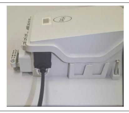
When shut, the lid compresses the seal to the cable.
