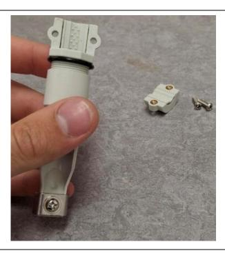
After unscrewing the halves, unscrew the gland body.
