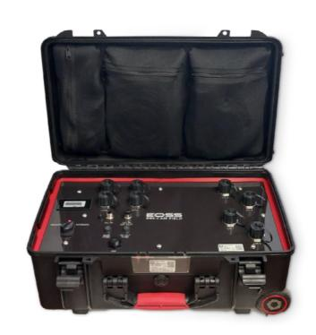
technology, the system can detect and classify PD without physical contact on the cable.
