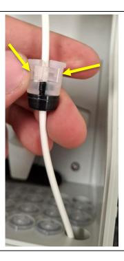
Place the rubber grommet and plastic housing around the drop cable. Click it shut.
