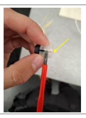
Then unclip the rubber from the plastic housing & open the plastic. The arrows show where the clips are to open it.
