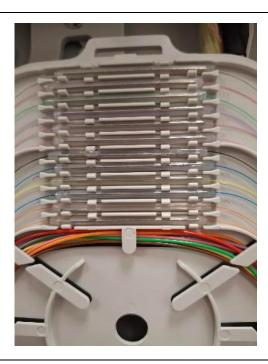
Splice the incoming cable to the existing pigtails, using your company's preferred method. Place the splices in the tray positions as shown.
