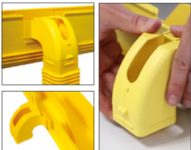
TC1279-89KIT Side drop-off to 50mm (2") square convoluted tube (TC1279 - 85YEL) - Can fit approx. 100-150 x 2mm cables - Also includes duct ramp
