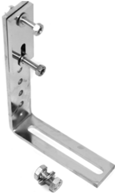
TC1279-155KIT Ladder-rack mount kit, 100mm and 220mm duct These clamps are a means of fixing either 100mm, 220mm duct systems to 1.5" and 2" ladder-racks Note: Used in conjunction with "C" type mounting hardware
