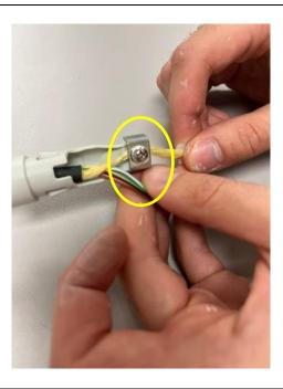
Feed your cable through the gland, anchor the aramid under the screw. Ensure that there is space under the metal and the screw is not fully tightened before trying to slot the aramid underneath it.
