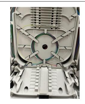
Splice the incoming cable to the existing pigtails, using your company's preferred method. Place the splice holder in the position as shown.
