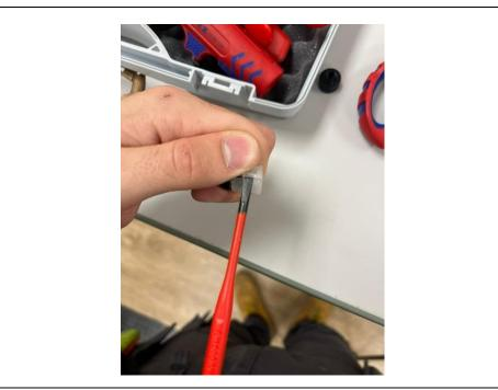
Then unclip the rubber from the plastic housing & open the plastic.
