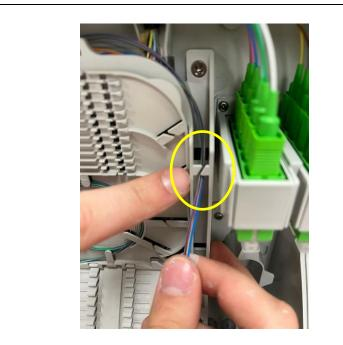
Bring the incoming cable elements on to the tray, ensure that they are stripped at the position pointed out.
