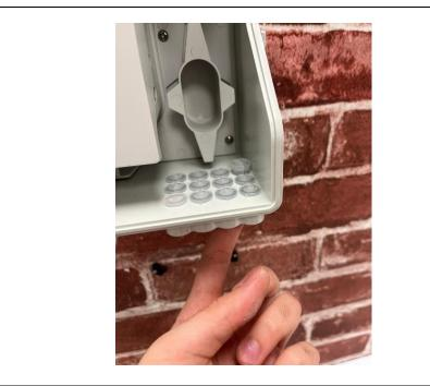
Push through the rubber grommet as shown. Then unclip the rubber from the plastic housing & open the plastic.
