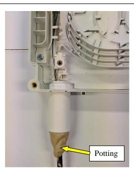
• If the port needs to be sealed, use local practices. The compound 16 can be used to block the end of port.
