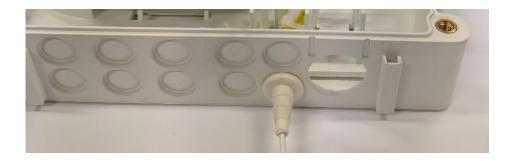
• The basement box is now ready to accept the installation and fibre routing of the output cables using the large knock out position. The 1 large port will accept the cables with a diameter of 4-9mm and 6-12mm.
