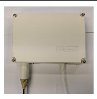
• Fit cover and tighten the 4 retaining screws.
