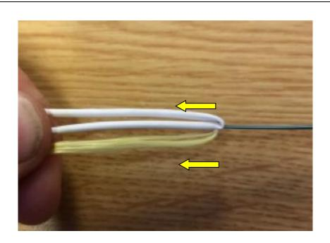
• Carefully fold back the sheath and separate the aramid strands as shown leaving at least 100mm.
