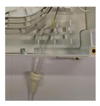
• Remove cable outer sheath to expose approximately 1.5m of fibre. Insert the cable through the Cable Grommet and into box.
