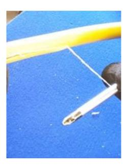
• Wrap the rip cord around a screwdriver and slit the sheath between the circumferential cuts. Remove element bindings and wrapping.
