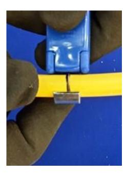
• Circumferentially cut the sheathing at the two marks using a stripper cable sheath 7 item code 126853.
