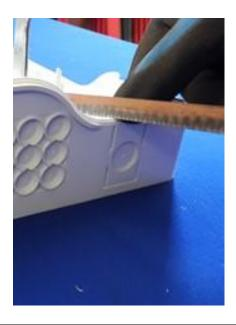
• Saw along moulded guides of the cable ports located at the top and bottom of the splitter DP.
