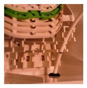
**Note:** The individual location of the cable anchor point within the closure is dependent on which row of cable ports the Customer Premise Cable enters from i.e. ports in rear row = lower anchor points.
