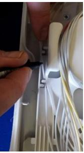
• Route the element containing the fibres to be spliced into the element guides. Mark the element at a position between the retaining tabs aligned with the centre of the loop storage manager.
