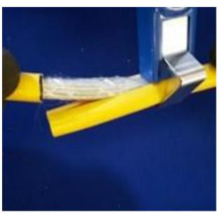
• At one of the circumferential cuts use the stripper cable sheath 7 to make a longitudinal cut of sufficient length to access a rip cord.
