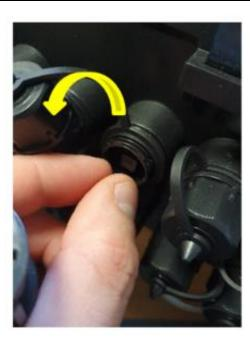
• Remove the MPO adapter blanking plug.
