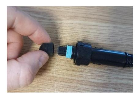
• Remove the MPO connector protective cap on the cable shroud.
