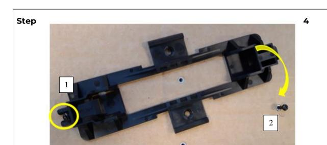
Slide the horizontal groove into position first, then rotate the bracket about the screw to fit the vertical groove over the second screw.
