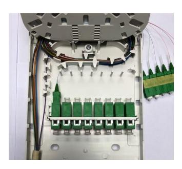
• Connect the SC connectors to the SC couplers by removing the protective caps.
