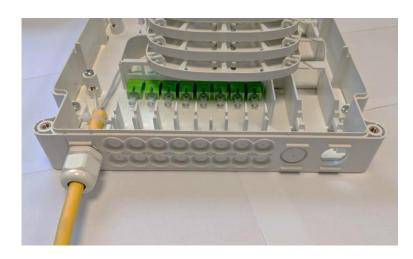
• Carefully knock out the cable entry port on the right-hand side of the base. Take care to support the base when doing this.
