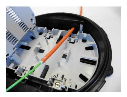
• Put the cable into the closure through the gland.
