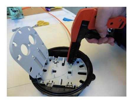
• Tighten the cable tie with a cable tie gun.
