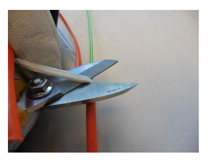
• Remove the cable out sheath and cut the strength element with scissor.
