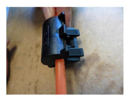
• Remove the mini duct with an Eden tube cutter from the second marker.
