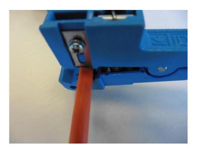
• Make a cut around the cable at the marker.
