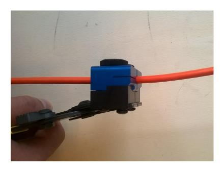
• Use Ripley stripping slitter to open the cable out sheath along the length direction, from the marker to the end of the cable.
