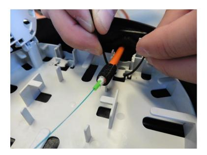
• Put a cable tie under the tab in the cable management plate.
