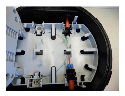
• Make sure fibres are routed inside the management plate as shown in the photo.
