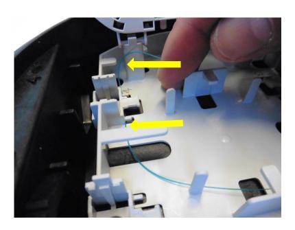
• Rout the fibre(s). Make sure they are under two small tabs at Port 4 (lower arrow in the photo) and behind the splice tray mounting support (upper arrow).
