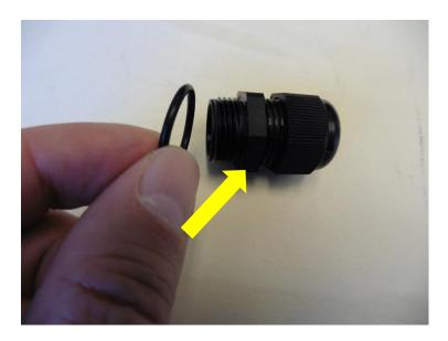
• Put O-ring onto the cable gland. Make sure the O-ring sit on top of the bottom surface next to the thread.
