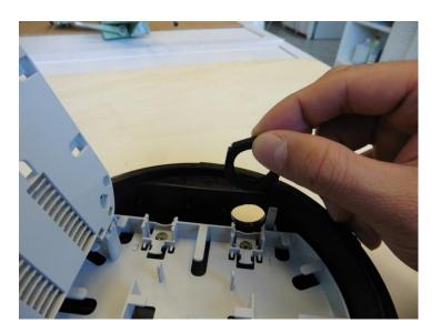
• Remove the cover and put lock nuts in the cable entry kit into the slots at the inner side of the closure body.
