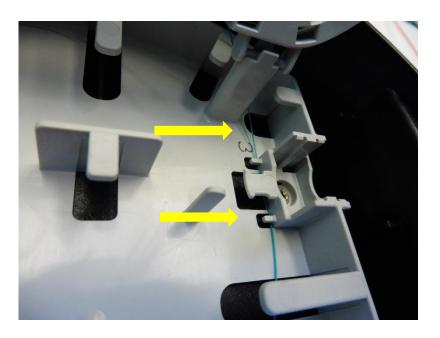
• Rout the fibre(s) under the tabs at port 3(lower arrow) and behind the splice tray mounting support (upper arrow).
