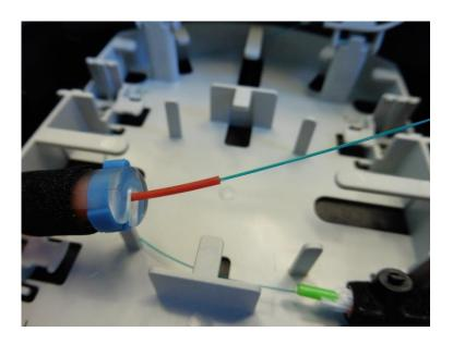
• Strip the out sheath of the fibre element and clean the fibre(s).
