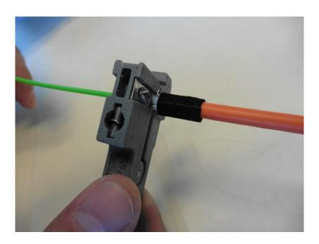
• Strip the fibre element sheath and clean the fibres.
