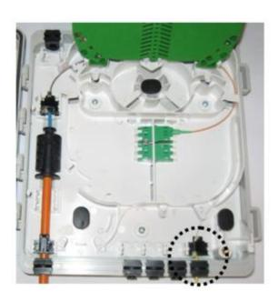
• Use the Cable Clips as described in the dedicated section. Install the cable clips with the right diameter on the Customer Cable in circled positions.
