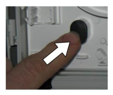
• Use the Oval Rubber Plugs to seal the three wall fixation points of the box.
