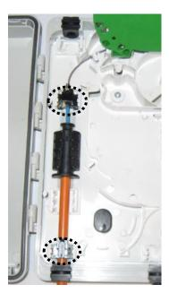
• Use the Cable Clips as described in the dedicated section. Install the cable clips with the right diameter on the tube and on the cable in circled positions.
