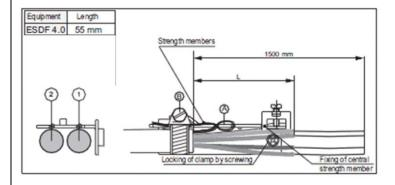
Cut the central strength members to 55mm and secure into bracket as shown.
