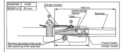
Cut the central strength member to 55mm and secure into bracket as shown.
