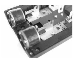
The joint has four cable entry ports, and a cable entry gland must be fitted into all four cable entry ports. In cases where only two or three cables are required to be installed, blank cable entry glands must be installed into the unused ports.
