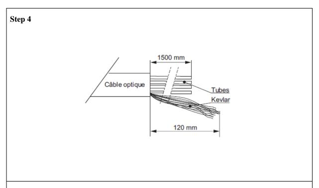
Mark the position of the cable butt at the port of the closure and strip the external sheath from the cable to expose 1500mm of the cable tubes. Cut away any excess cable length.
