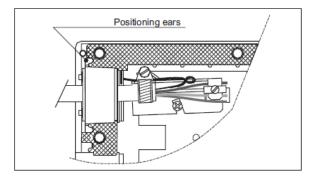
Slip the seals along the cable and seat them into position in the closure body. Ensure that the ears on the seal fit properly within the corresponding cut-outs in the flat seal.
