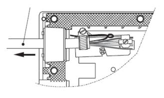
To remove a cable, slip the seals along the cable using grease if required.
