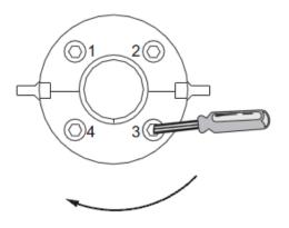
Tighten the seals in the order shown on the diagram opposite. Execute a maximum of two turns per screw before moving to the next screw.
