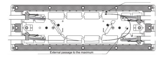
It is possible to route the fibres from the cable tubes through protective spiral wrap tube.
