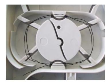
• Route the first 12 fibres around the tray once in preparation for splicing.
