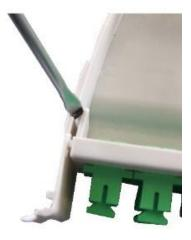
• To remove a uniter panel, press the two tabs (one either side) and pull the uniter panel forward. (Ensure there are no pigtails connected to the uniter panel before you remove it).
