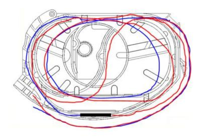
• Splice the fibres to the pigtail fibres already stored on the splice tray.
