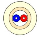
Semi-tight optical fibre: coloured 900µ semi-tight buffered BendBright<sub>®</sub><sup>xs</sup> fibre. Easy strippable. Reinforcement and protection: dielectric yarns. Outer Sheath: LSZH-FR material.
