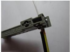
Apply a circumferential cut to the loose tube at the cable butt
