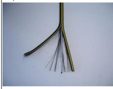
Separate the two halves of the Fibre Drop Cable sheath back to the mark made in step 25.
