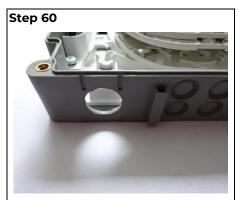
Carefully knock out the cable entry port on the left hand side of the base. Take care to support the base when doing this.
