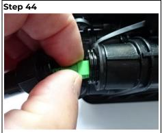
Push SC connector into the adapter. Ensure locating the rib is facing upwards to line on top of the port.
