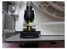
Secure the cable with cable tie in position shown.
