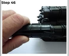
Using the CBT Connector Tool tighten the shroud nut fully.
