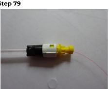
Attach the connector onto the locking tube.
