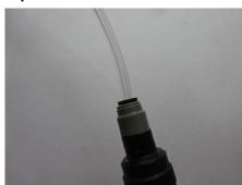
Fit the tube to the reducing connector.
