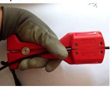
Pull the cutter along the cable. WARNING: Failure to maintain the 90° position relative to the cable wire strength members may result in permanent damage to the stripper tool.
