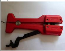
Open the cutter by pulling down on the black arm.
