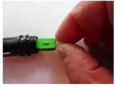
Remove the SC connector protective shroud.
