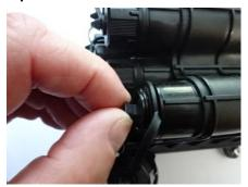
Remove the adapter blanking plug. Note: The colour may differ.
