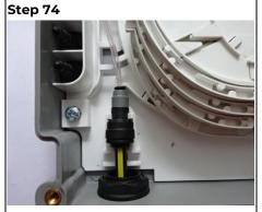
Locate the completed tube assembly into position and clip the connector into place.
