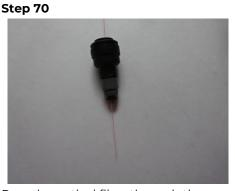
Pass the optical fibre through the 6mm – 3mm connector.
