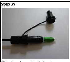
Slide the shroud body back. Do not pull against the connector.
