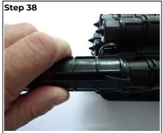
Using the CBT Connector Tool remove the cap from the relevant port on the CBT. There is a number by the port for identification.
