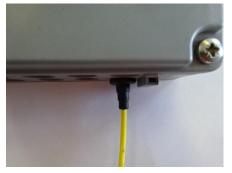
The output cable can be fed through the gland and the optical fibre spliced onto the drop cable fibre.
