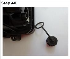
The CBT Port Cap retaining straps on the Pulling Eye can be removed if required but the rubber washer must sit under the cable nut.
