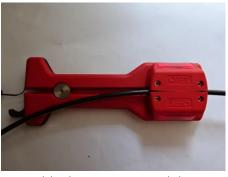
Assemble the cutter around the cable at the mark made in step 24. The blades should be positioned over the groove and yellow line.
