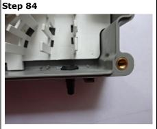
Fit the output gland into the enclosure.
