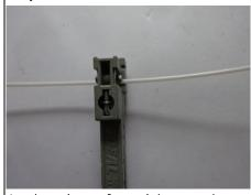
Apply a circumferential cut to the loose tube at 1m from the end of the tube.
