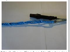
Attach the pulling bond to the tension clamp.
