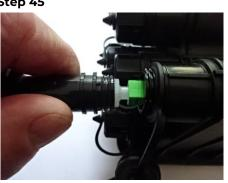
Line the rib on the shroud body to rib on the port and insert the shroud into the port.
