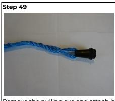
Remove the pulling eye and attach it to the pulling bond.
