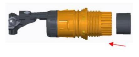
• Align the 3-way seal with the gland body assembly.
