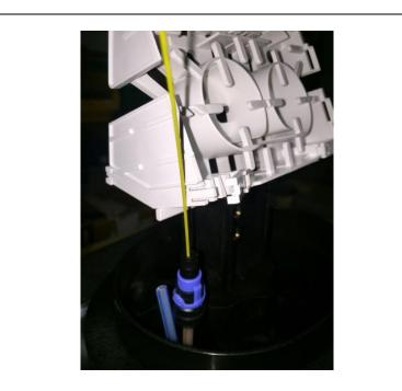
• Feed a water block connector (BT Item Code - 006848 Blown Fibre Tube 5mm to 3mm water block connector) over the fibre unit and plug onto the tube.
