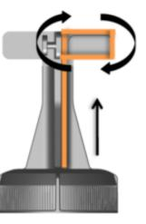
WHILST KEEPING TENSION ON THE CABLE, BEGIN TO WRAP THE ARAMID AROUND THE ARAMID CHANNEL STARTING FROM THE INSIDE TO OUTSIDE UNTIL A MINIMUM OF 1.5 TO 2 TURNS HAVE BEEN MADE.
