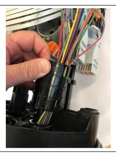
• Slide the tool over the gland and push into the base. When clips disengage remove gland from base and carefully pull out all tubes and fibres.
