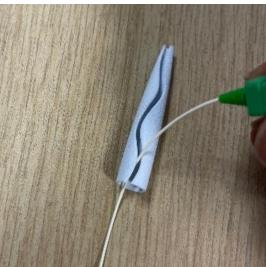
For ease of routing fibre along the RACEWAY, first route the fibre into Cable Placing Tool.
