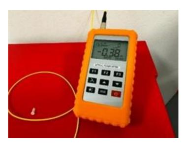
A final optical test must be carried out to ensure connectivity across the installation.
