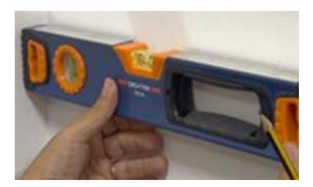
To have a precise path on surfaces with no edges and corners, using a spirit level, lightly mark a straight line on the wall with a pencil.
