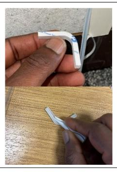
To pass the RACEWAY around a corner, please use the Planar Corner Tool.
