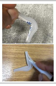
To pass the RACEWAY around an external corner, please use the edge corner tool.
