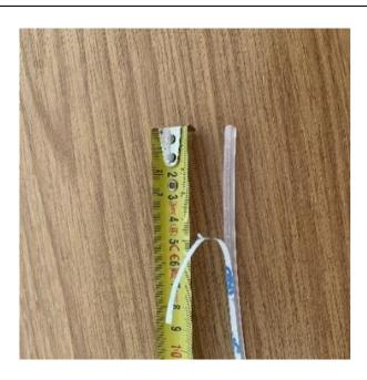
To commence installing the RACEWAY, take off 5cm of the protective liner.
