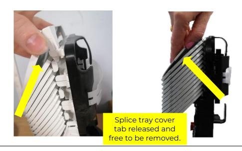
• With the other hand slide your thumb and fingers underneath the tab.
