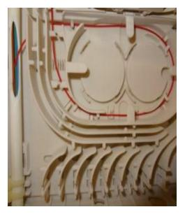
• Route the fibre element into the input channel, around the locking area.
