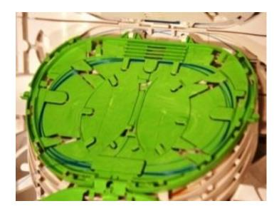
**Note:** The Splitter device input fibres are pre-installed into the (green) device tray such that the nominated working fibre (blue) is in TR AY 1.
