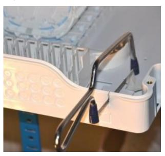
• Remove BFT port cut-out located on the top and bottom of closure using a suitable hacksaw.
