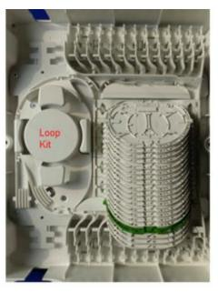
• Install the Loop Kit item code 063238 using the two mounting screws provided.
