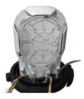
Install the drop cable into the port and lock the CSM into the anchor bracket by tightening up the Screw.
