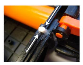
REMOVE THE EXCESS LENGTH OF FOAM CORD AT EACH OF THE FOUR POSITIONS USING SCISSORS TO CUT IT FLUSH WITH THE TOP SEALING RIB.
