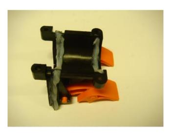
TAKE THE IN-LINE CLAMP AND APPLY A CONSTANT BEAD OF SILICON DOWN EACH SIDE AND CONTINUE INTO THE SEALING RECESS.
