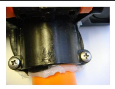
WHEN ALL SCREWS ARE FULLY TIGHTENED IT IS NORMAL TO SEE EXCESS SEALING TAPE AND SILICON SQUEEZED OUT AROUND THE SEALING AREAS BOTH INSIDE AND OUTSIDE THE BOX.
