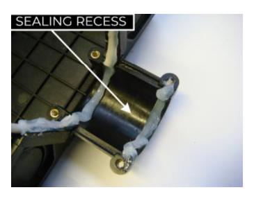
APPLY A CONSTANT BEAD OF SILICON DOWN THE FOAM CORD AT EACH SIDE AND CONTINUE INTO THE SEALING RECESS.
