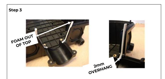
TAKE THE FOAM CORDS AND PUSH THEM FIRMLY INTO THE GROOVES LOCATED AT THE CABLE ENTRY POINT. DO NOT DRAG OR PUSH THE FOAM WITH A SHARP INSTRUMENT AS THIS WILL AFFECT THE SEAL INTEGRITY.
