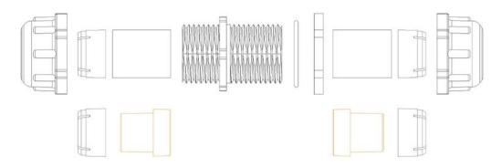
**NOTE:** ONLY XBFSC00220 8mm – 11.5mm CABLE GLAND KIT CONTAINS 4 RUBBER SLEEVES AND 4 UPPER WASHERS. ALL OTHER KITS CONTAIN 2 RUBBER SLEEVES AND 2 UPPER WASHERS
