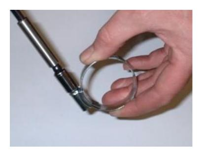
• Repeat steps 7 and 8 on each of the drop ports being used. Then tighten down all the jubilee clips.
