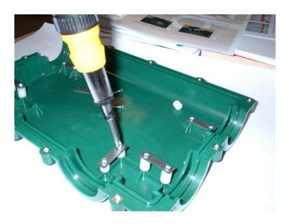
• Use the remaining spacers and screws to assemble the clamping plates at ports 4 and **Note: If not window cutting** (intercepting) go to step 5.
