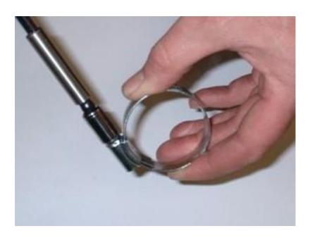
• Separate the large jubilee clips by undoing the screw until the two halves come apart.
