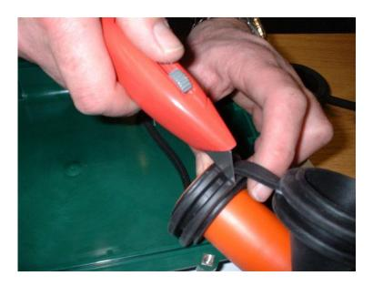
• If window cutting use the knife to remove the cones from ports 1 & 2, using a 'dummy' section of 24-way assembly cut both straight grommets as shown above. If using 19 way or 7-way DB use the rubber spacers provided.
