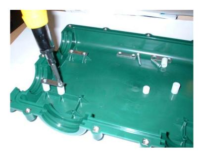
• Using the largest spacers and screws build the clamping plates at ports 3 and 6.
