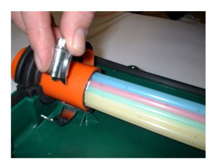
• Place the opened jubilee clip around the assembly and under the clamping plate, then re-tighten. Repeat for the other side of the assembly.
