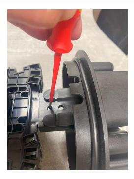
• Using a flat-head screwdriver, gently push the tab out through the hole in the base. When pushing the tab pull the spine away from the base.
