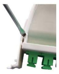
• To remove a uniter panel, press the two tabs (one either side) and pull the uniter panel forward. (Ensure there are no pigtails connected to the uniter panel before you remove it).
