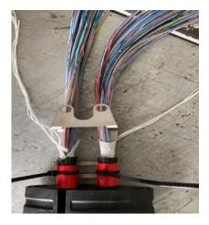
• Slide the metal plate along the cables and fix the cable ties at 16mm from the cable butt ends.
