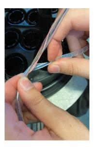
Begin spiral wrapping the cable to protect the fibres.
