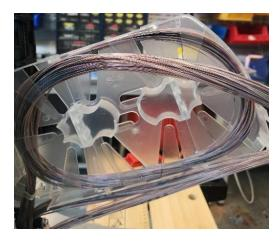
• Route the elements around the outside of the mid span loop manager in a clockwise direction.
