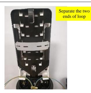
• Firstly, separate the two ends of the loop. Gently straighten the loop away from the MMJ ready to loop into the spine.
