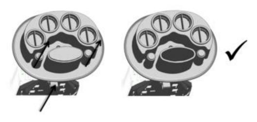
• Knock out the oval port end plate of the Joint from the inside using a large screwdriver and remove any burrs using a file.
