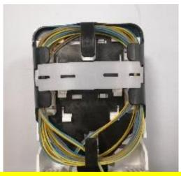
A single loop should be remaining after several coils have been installed.
