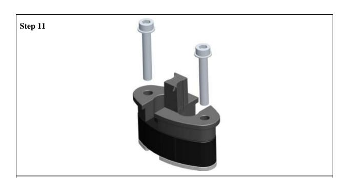
• Insert washers and screws and lightly screw together.
